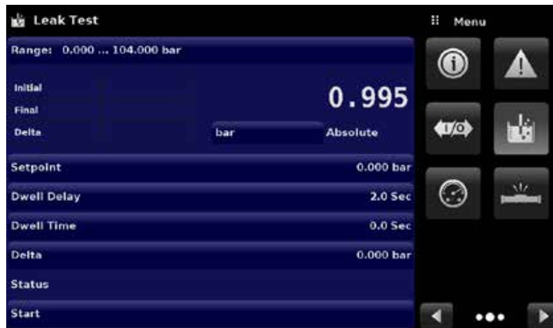
Figure 6.4.12 Leak Test App
