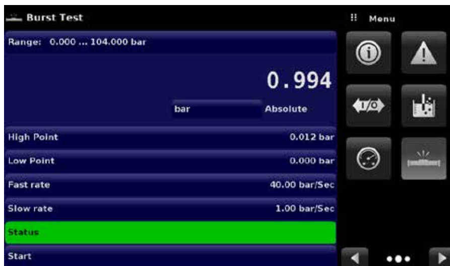
Figure 6.4.14-B Burst Test Complete (No Burst)
