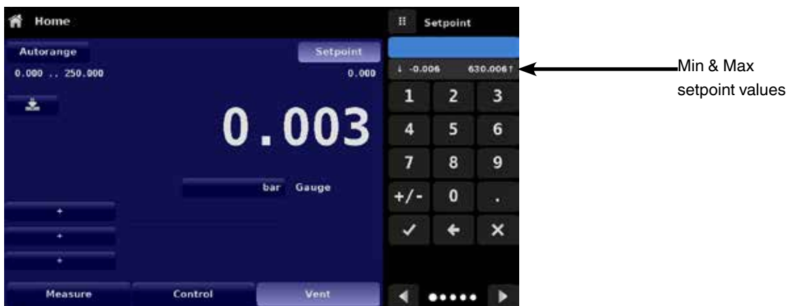
Figure 6.4.1.2.1 Numeric Keypad Setpoint Entry
